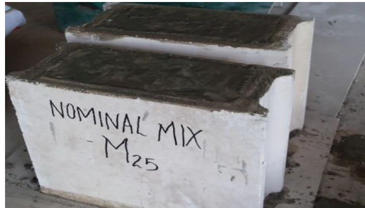
Fig.1. Modular cavity of panel filled with nominal M25 mix concrete
