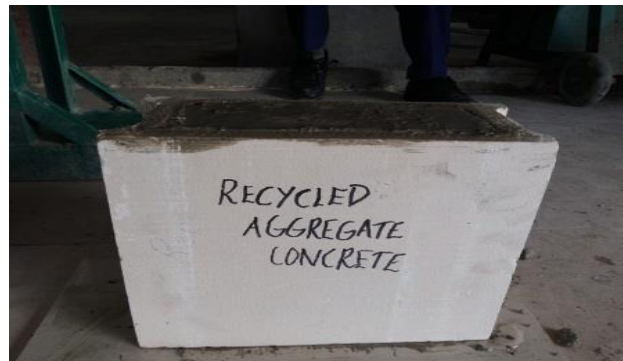
Fig.3. Modular cavity of panel is filled with recycled aggregate concrete
