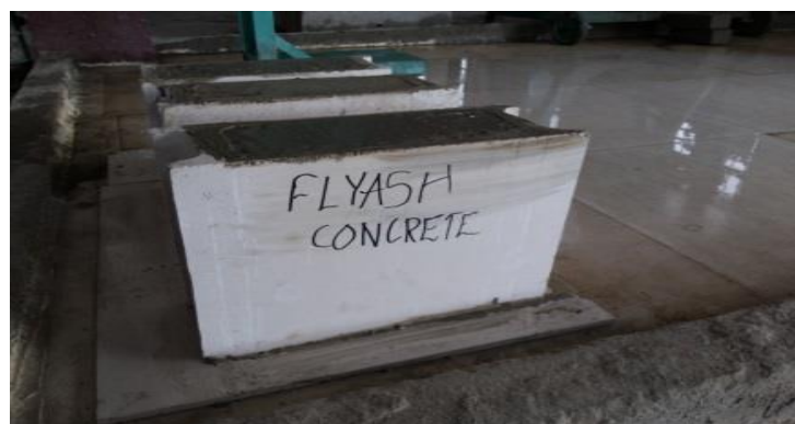
Fig.2. Modular cavity of panel is filled with flyash concrete
